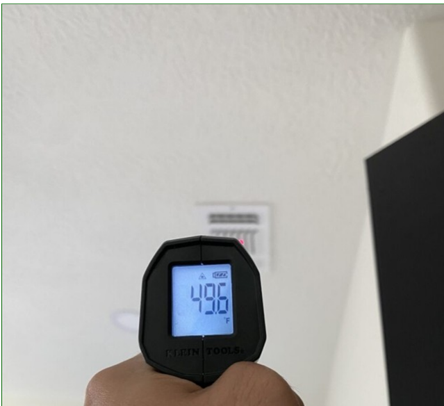
B. Item 2 (Picture) Master bedroom, HVAC supply vent, A/C supply temp. reading
