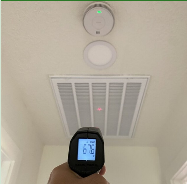
B. Item 1 (Picture) Hallway, HVAC return vent, temp. reading
