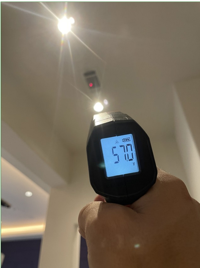
B. Item 6 (Picture) Common area, A/C supply vent, temp. reading
